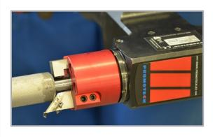
Extension set for pipes from ID 42 mm (1.65") up to 0D 60.3 mm (2.37") Product Code:
