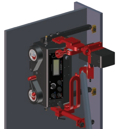
Fillet Welding with oscillator
