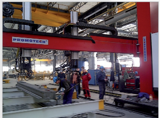
Half Gantry Beam and Tank Welding System C&B type WA with LINCOLN ELECTRIC PW AC/DC 1000 SD
