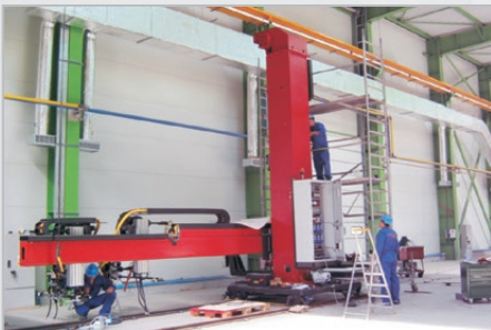
Installation and commissioning of Column&Boom at the customer's site
