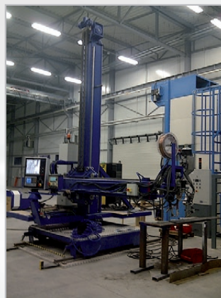
Standard Column & Boom with ESAB Aristo 1000 AC/DC
