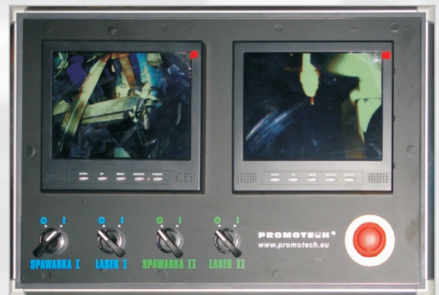
Optional equipment includes: camera system for GMAW/SAW, automatic correction of welding gun position or remote control.
