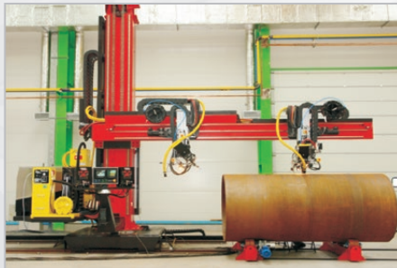
Installation and commissioning of Column&Boom at the customer's site
