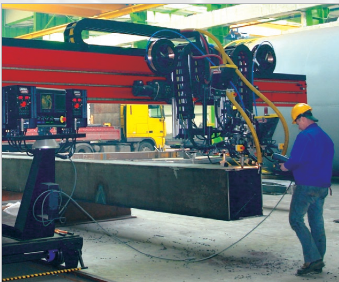
Standard Column & Boom with ESAB Aristo 1000 AC/DC
