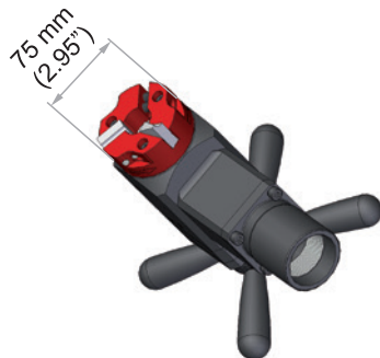
Minimum distance between tubes is 75 mm (2.95")
