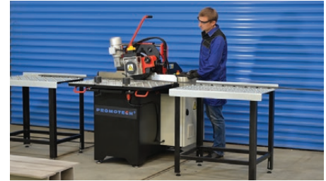
Auxiliary tables to accommodate long workpieces
