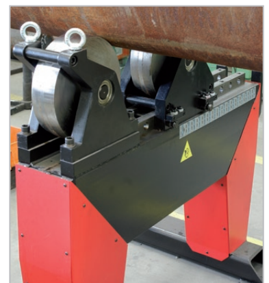
Heavy-duty adjustable pipe support ( \varnothing 200-1000 mm)
