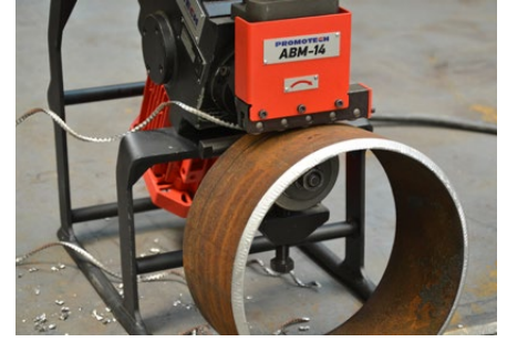
Oval workpiece and pipe beveling
